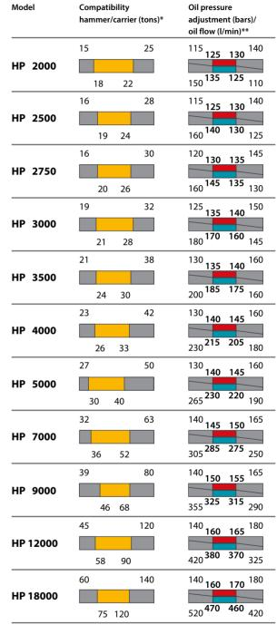
\*Suggested uses on machines with an overall weight (in tons):
